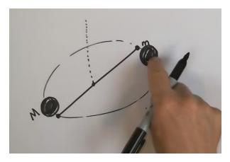
Cavendish used an experiment where two small lead spheres were fastened to the ends of a rod which had a very fine string (actually a quartz fiber) attached to the middle so it could be lifted off the ground. This is called a torsion balance, meaning that you can carefully measure the twist in the string by measuring how much the rod spins around. (Torsion balances can be made from other materials that have a stiffer spring constant value, like metal rods.)
